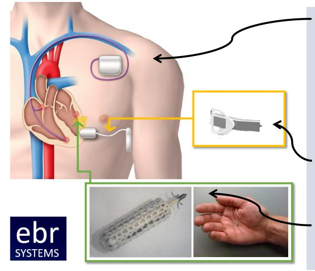
Conventional Device ("Co-Implant") Provides RA and RV Pacing (Pacemaker, ICD, CRT-p, CRT-D)
