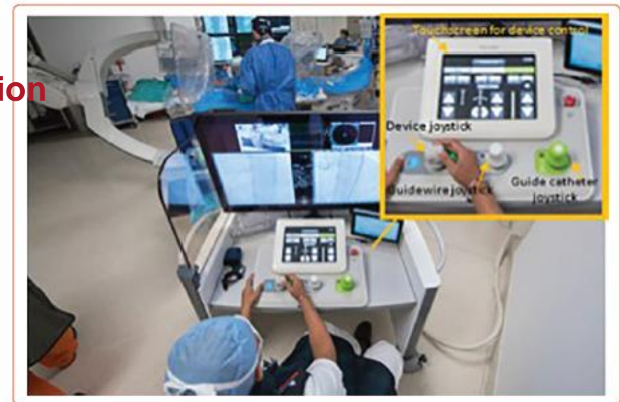
Figure 1: Robotic Percutaneous Coronary Intervention in the Cleveland Clinic Catheterization Laboratory
