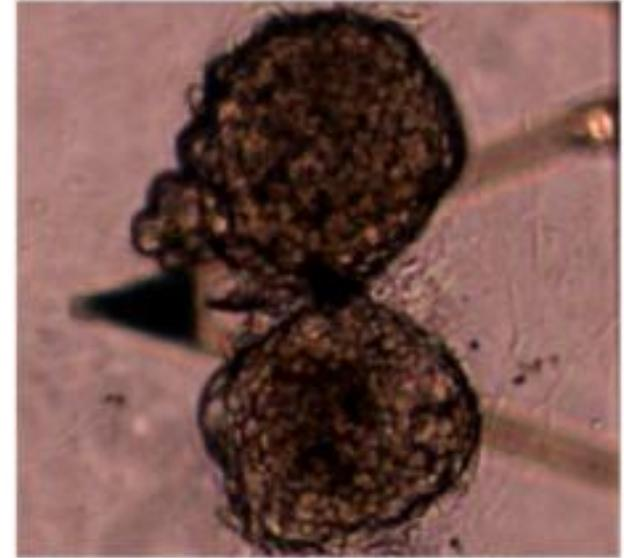
Atomic Force Microscope biosensor using couples cardiac organoid twin structure
