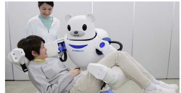
Assistive technologies: robots that can lift and carry to compensate for disabilities – RoBear, Japan
