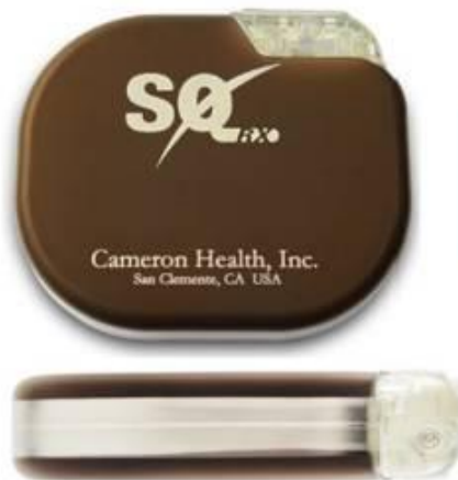
1st generation S-ICD SQ-RX 1010 (Cameron Health)
